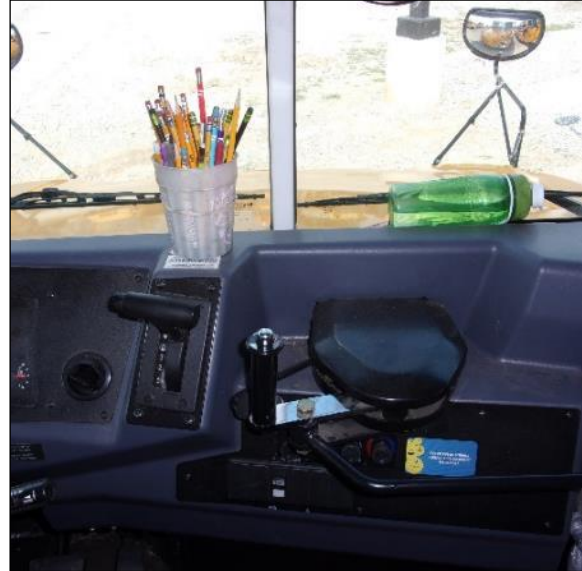
Bus 62 – Driver's Window Obstructed
